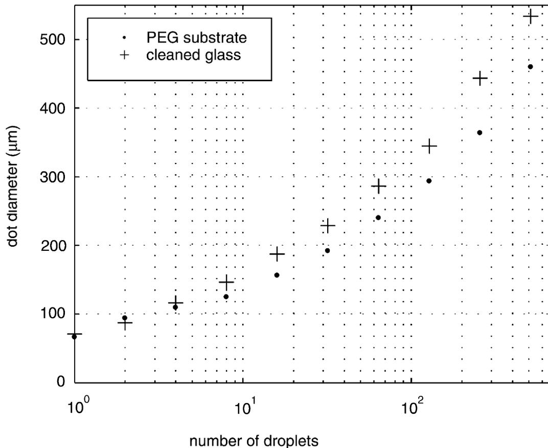
Fig. 5. Micro-island size scales with droplets deposited. For each data point, the ink-jet print head was placed at a single  $X$ – $Y$  location and multiple droplets were deposited in quick succession (500 Hz) so that they were all deposited before any significant drying had occurred. The diameter of a micro-island grew slowly as the number of droplets deposited increased and also depended on the composition of the substrate being printed onto ( $n = 8$ ).
